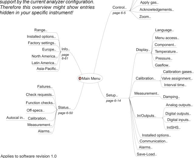
Fig. 6-1: X-STREAM Software Menu Structure
